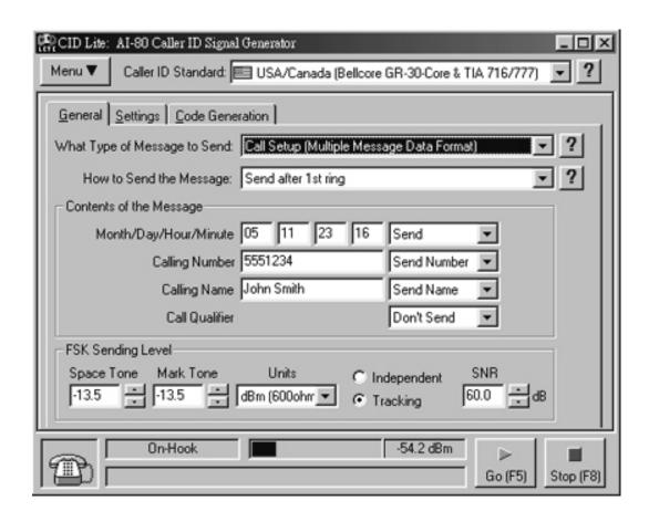
The CidLite program works in conjunction with the AI-80 Caller ID Signal Generator to provide a simple means for generating the caller ID signals specified by various standards and specifications in use today. This includes both the Bell 202 and V.23 FSK data transmission standards, as well as the DTMF based standards. The CidLite provides an easy to use software interface for the AI-80 so that it is not necessary to develop an application program for the most common Caller ID Standards.
