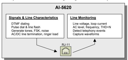
The wide range of programmable line characteristics gives the AI-5620 the ability to present conditions that fall both inside and outside the conformance range of various standards. This helps to ensure that the equipment being tested can experience conditions outside the normally expected range.
