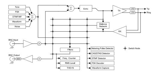
The AI-5620 has three primary signal sinks. They are a signal measurement meter, signal analyzer, and the rear panel BNC output connector.
