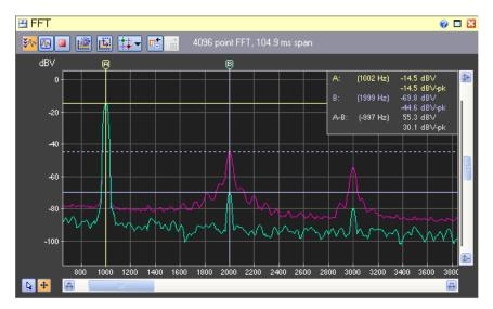
4. Viewing a real time FFT of a 1 kHz tone. The purple trace represents the peak hold channel, which shows the effect of transient conditions. The two cursors are used to measure the second harmonic level of the 1 kHz tone. In this case, the second harmonic is normally 55 dB lower than the fundamental tone; however a transient event recorded by the peak hold dramatically increased the harmonic level by approximately 25 dB.
