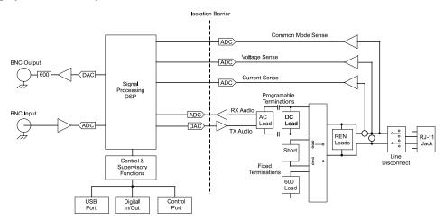
At all times, the AI-5620 monitors and records the metallic line voltage, common mode voltage, and loop current. Measured AC signals are processed for the detection of a wide range of telephony related events such as DTMF digits, Caller ID FSK messages, CAS/DTAS, or metering pulse tones.
