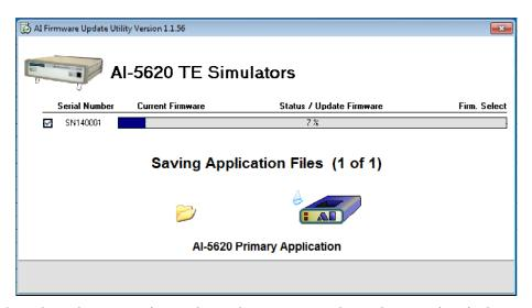
Once the update process is complete and no errors were detected, a green icon is shown to the left of the device information. If the update could not be completed due to errors, a message providing information on the error is displayed. Please contact us for assistance in resolving the error.
