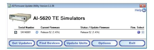
The check box to the left determine which devices are to be updated. By ensuring it is checked and clicking on the **Update Units** button, the process of installing the selected firmware begins.
