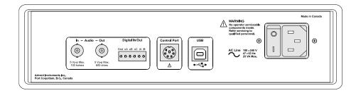
The BNC output connector can be used to monitor signals from the telephone line as well as other internal signal points. Its output impedance is  $600~\Omega$  with a maximum output level of 5 Volts peak-to-peak. The BNC input connector is AC coupled and accepts a maximum peak-to-peak signal of 5 volts. Its input impedance is  $100~\text{k}\Omega$
