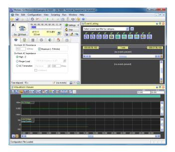
The window is itself divided into sub-regions, termed 'views'. In the example above three views are present. They are the 'Status & Action' view located in the top left corner, the 'Event Listing' shown in the top right corner, and the 'Waveform Viewer' located along the bottom of the window.
