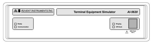
After a short duration all the indicators except for Ready will turn off. The AI-5620 then waits for the PC to recognize its connection via USB. While waiting, the Ready indicator flickers once every second.
