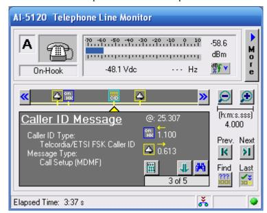
The top portion of the window displays the current line status and signal level. Both AC RMS level and DC line voltage are shown. AC signal frequency is displayed if sufficient signal level is present. Options exist to apply various signal filters (adjustable low pass, high pass, band pass, and notch) in order to minimize unwanted or interfering tones.
