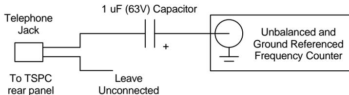
Note: In this setup, if the frequency counter and PC that contains the TSPC are ~~not~~ properly connected to earth ground, a large amount of 50/60 Hz hum noise can effect the measurements.
