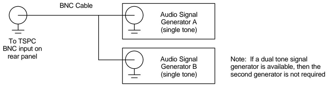
It is also important that the meters and frequency counters used have balanced and floating inputs. If this is not the case, then the CID1500 will display "line unbalanced", indicating the lack of balanced floating inputs on the test equipment. While most meters have balanced floating inputs, it may be more difficult to locate a frequency counter with a balanced floating input. However, most often the audio signal meter includes the capability to measure signal frequencies.
