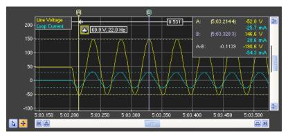
When either cursor is displayed, the top right corner of the graph displays the time position of each cursor along with the reading of each waveform channel the cursor passes through. In the example above, cursor 'A' is positioned at a minimum ringing voltage and current, while cursor 'B' is at a corresponding maximum two and a half cycles later.
