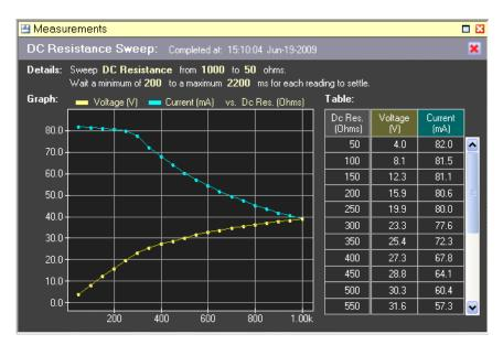
In the above example, the resistance was swept from 1000  $\Omega$  to 50  $\Omega$ . As the resistance is reduced, the line voltage decreased and the loop current increased.
