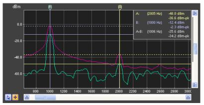
When either cursor is displayed, the top right corner of the graph displays the frequency position of each cursor along with the reading of the current FFT results and the peak detector (if enabled). In the example above, the 1 kHz tone indicated by cursor 'B' has a peak level of -36.6 dBm and is currently reading a level of -48 dBm. The harmonic at 2 kHz is approximately 36 dB lower in level.
