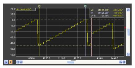
When either cursor is displayed, the top right corner of the graph displays the time position of each cursor along with the measurement reading for each channel present. Since each channel records both the minimum and maximum readings during the sample interval (approximately 200 ms), the value reported by the cursor is the average of these two readings.
