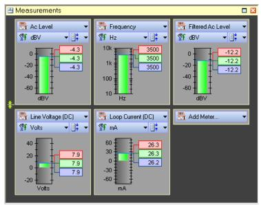
By clicking the mouse on one of the three buttons, a popup menu appears listing the available selections. The measurement type includes 15 different reading types for AC signal level, AC signal frequency, line voltage, loop current, tip lead voltage, ring lead voltage, and common mode voltage.
