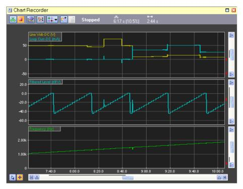
The above figure shows an example of the chart recorder view. Each view can display from one to four graphs, with each graph containing different (or the same channels). In the example above, the top most graph plots the measured DC line voltage and loop current. The middle graph plots the filtered AC signal level in units of dBV, and the bottom graph plots the AC signal frequency in Hz.
