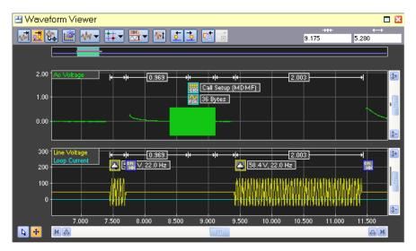
Each waveform view includes a tool bar of common operations (shown at the top), a time line of captured waveforms (below the tool bar), and finally one or more waveform graphs. In the example above, two graphs are displayed. The top most is configured to show the AC coupled line voltage (green trace), while the bottom most shows the captured DC coupled line voltage (yellow trace) and DC coupled loop current (blue trace).
