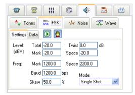
The **Skew** setting controls the bit time skew between the mark bit and the space bit. It is defined as the ratio of the mark bit time to the sum of the mark and space bit times. A value of 50% indicates equal bit time periods.
