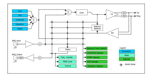
The **Meter Source** selection controls where the AC level, frequency, and THD+N meters obtain their signal for measurement. This setting effects the broadband level meter shown on the 'Status & Action' panel, as well as the measurements used by the AC signal sweeps and the chart recorder.
