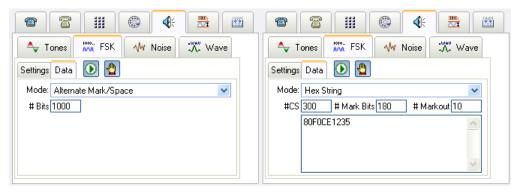
To start the FSK generator, click the 'Start' button located next to the 'Data' tab. Stopping the generator is accomplished by clicking the 'Stop' button.
