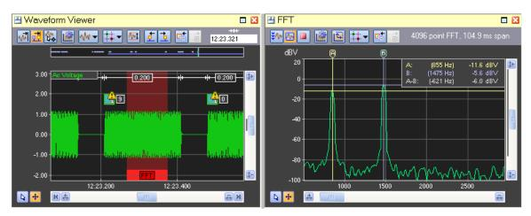
The waveform view highlights in a red background color the time range used for the FFT calculation. Its position is always fixed to the center of the graph, while its width is determined by the number of sample points used to calculate the FFT. The number of sample points used in the FFT calculation is controlled from the graph settings window.
