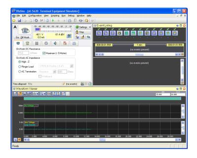
The window is divided into sub-regions, termed 'views'. In the example above three views are present. They are the 'Status & Action' view located in the top left corner, the 'Event Listing' shown in the top right corner, and the 'Waveform Viewer' located along the bottom of the window.
