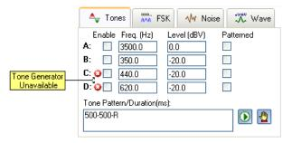
Tones that are currently in use are indicated by a small red 'x', as shown in the above figure. Hovering the mouse on top of the red 'x', displays the reason the tone is unavailable.
