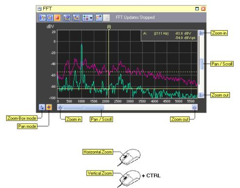
A tool bar at the top of the view provides access to various graph settings and FFT related functions.
