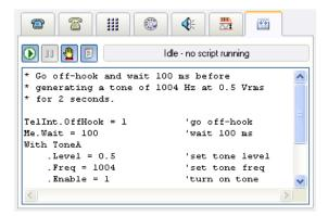
Controlling the execution of a script is performed by using the three buttons shown in the upper left corner. Clicking the start button downloads the script to the AI-5620 and starts its execution. While the script is running, clicking the pause button suspends execution indefinitely. To resume operation, click the start button. Finally clicking on the stop button terminates the script program immediately.
