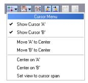
Two cursors, labeled 'A' and 'B' may be displayed or hidden by selecting the 'Show Cursor' menu commands. When first displayed, the cursors are positioned in the center of the waveform graph.
