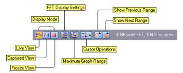
Clicking the 'FFT Display Settings' button displays a window with various settings that control the FFT processing. This includes options to compute FFT averages and perform peak hold functions. See the following section for details on the various settings contained within this window.
