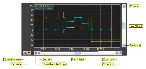
Zooming in or out the graph's horizontal range is easily performed by rolling the mouse wheel up or down. Rolling the mouse wheel up performs a horizontal zoom 'in' at the current position of the mouse, while rolling the mouse wheel down performs a zoom 'out'.
