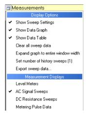
The TRsSim software remembers the last twenty AC signal sweeps performed. The results from earlier sweeps may be viewed by using the 'Next' and 'Previous' buttons located in the upper right corner of the view. Clicking on the right most 'Erase' button deletes the data from the currently viewed sweep.
