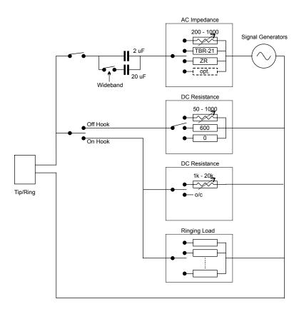
The AC impedance terminations may be connected to the tip/ring leads in both the onhook and off-hook state. However the default setting disconnects them in the on-hook state.
