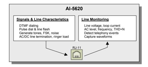
Both functional blocks generally operate independently from each other. If the line settings are placed in a high impedance state, the AI-5620 will simply monitor the telephone line making measurements and listening for telephony related events such as ringing, dialing, Caller ID, metering pulses, among others. Only when the AI-5620 presents an AC termination can it generate signals such as DTMF, FSK, or other AC signals.
