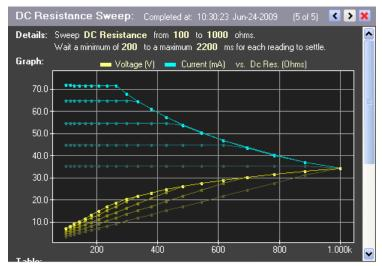
Depending on the source mode selection, the graph's horizontal scale will be in units of ohms, volts, or mA. In all source modes, the graph always uses a linear scale in both the vertical and horizontal axis.
