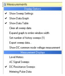
The common mode voltage measurements are by default not displayed. They can be shown by selecting the appropriate command from the view menu shown above.
