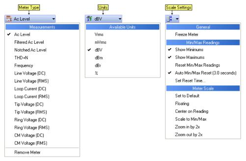
By default, each meter displays a maximum and minimum reading that resets once every 3 seconds. To change the display of the peak readings or change the reset time, click the scale settings button. Other scale options include changing its center position, allowing it to float, or changing the range of the scale.
