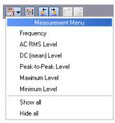
Waveform measurements are performed only over a limited time range. This range can be adjusted from a minimum of 10 ms to a maximum of 30 seconds. When a long time range is used, the measurement may take a few seconds as a large number of waveform samples must be processed. If at least one measurement type is enabled, the time range used is displayed just above the waveform graph as shown in the following figure.
