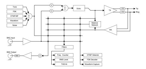
The AI-7280 has three primary signal "sinks". They are a signal measurement meter, signal analyzer, and the BNC output connector.
