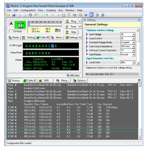
The TRsSim software supports a variety of testing functions. Its ringing generation is programmable over wide range of level, frequency, and cadences. Network tones such as dial, stutter dial, ring back, and busy are predefined, and user defined tones can include arbitrary levels and frequencies or be composed of DTMF and MF tones. Supported MF tones include both the ITU Q.320 and Q.441 variants.
