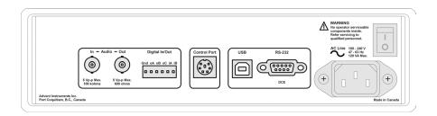
The two BNC connectors can either monitor various signals internal to the AI-7280 or inject signals into the AI-7280. The BNC input connector is AC coupled and withstands a maximum DC voltage of 55 volts. It can accept a maximum peak-to-peak signal of 5 volts with an AC input impedance of 100 k  $\Omega.$  The BNC output connector is DC coupled and outputs a maximum of 5 volts peak-to-peak with an output impedance of 600  $\Omega.$
