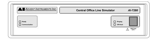
A number of checks are performed during the power up cycle. If a fault is detected, the "Ready" indicator will either flash or be off. If it stays off, the fault is serious and requires that the unit be returned for repair or replacement. In either case, see Appendix B: Error Codes for more information.
