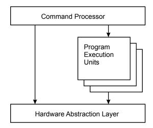
Starting from the bottom of the figure is the Hardware Abstraction Layer (HAL). This is simply a layer of software that controls all hardware related aspects of the AI-7280. The AI-7280 functionality is represented by over 200 properties. These properties are organized into groups of similar function. The groups control various settings, such as the ringing generator, tone generators, level meters, FSK modulator, FSK generator, DTMF detector, and others.
